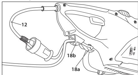
To secure the supply (connecting) cable, this chainsaw is equipped by strain relief (18). At first connect the power cord plug of the device (12) with the supply cable. Create a loop on the connecting cable and push it through the bridge (18b) on the bottom device side. Hang the loop on the hook (18a). The connecting cable is thus secured from undesirable spontaneous disconnection.
