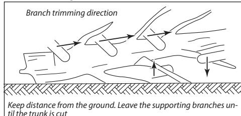
Branch trimming is understood separation of branches from the fallen tree. When trimming, leave at first the larger branches supporting the trunk. Trim smaller branches by a single cut. The sprung branches should be cut from bottom to top to avoid chainsaw jamming.
