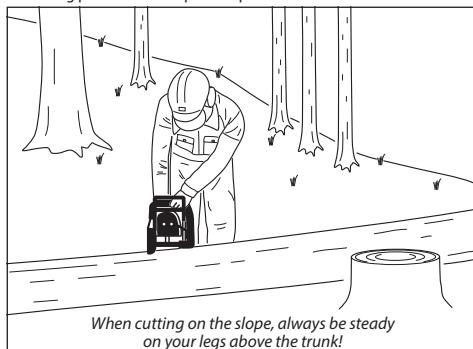
When cutting on the slope, stay as shown in the Figure. To have a full control over the chainsaw at the moment of full cross-cut, reduce the pressure in the final cut phase, still holding chainsaw handles firmly in your hands. **Attention, the chain may not touch the ground!** When the cut is complete, wait until the chain is stopped and only then take out the chainsaw.
