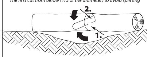
If the trunk lies on the ground by its one end, see Figure, cut at first 1/3 of trunk diameter from the bottom side and then the remaining part from the top as deep as the bottom cut.
