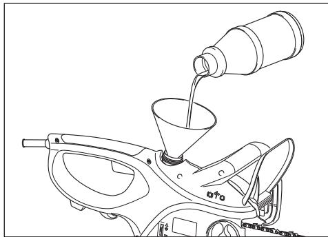
**Attention! Be so kind and use only the oil suitable for the saw chains, on the biological basis and 100% degradable.**
