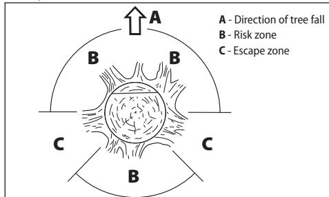
Prior to start cutting, the escape route should be planned and cleared, if necessary. The escape route should lead obliquely from the expected falling tree track, as can be seen in the Figure.
